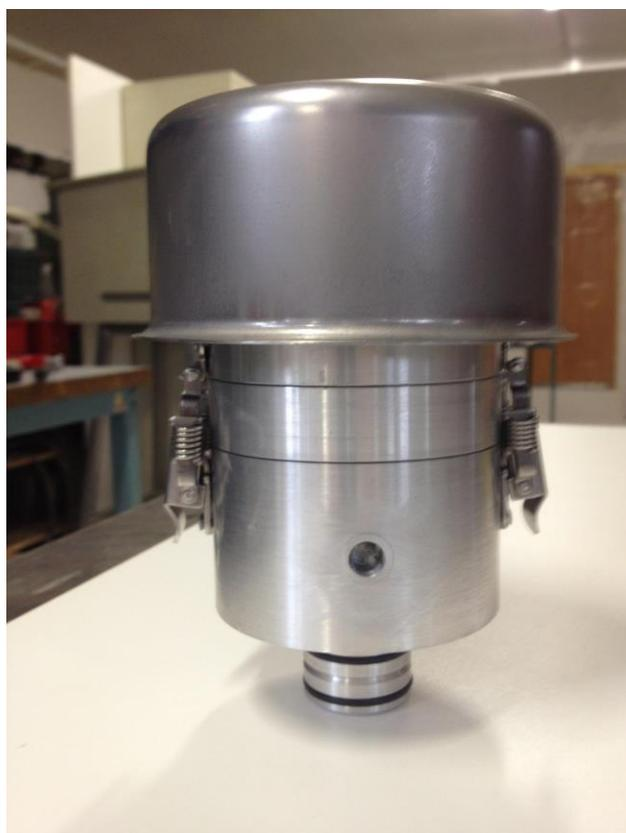
**Advantages/Benefits:** Filters are replaced inside the laboratory in an appropriate working environment. This removes the problems caused by changing the filters in the open air (e.g. wind, rain, etc.). This reduces the risk of compromising the analysis results. The alarm system ensures more easy and efficient operation of atmospheric dust sampling due to the fact that faults are identified and communicated immediately.
