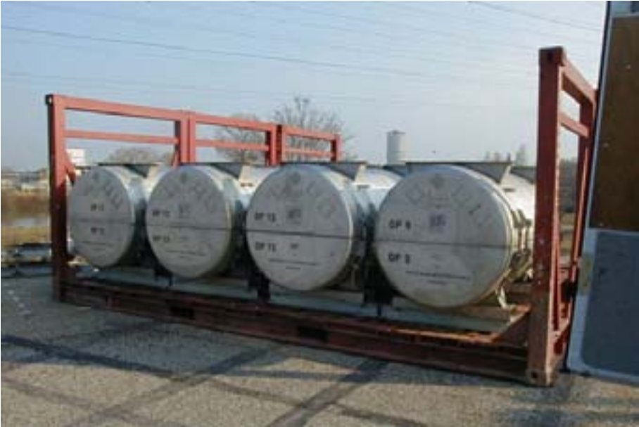
FIG. 15. Casks used for the transport of enriched uranium hexafluoride from enrichment facilities to fuel fabrication facilities.
